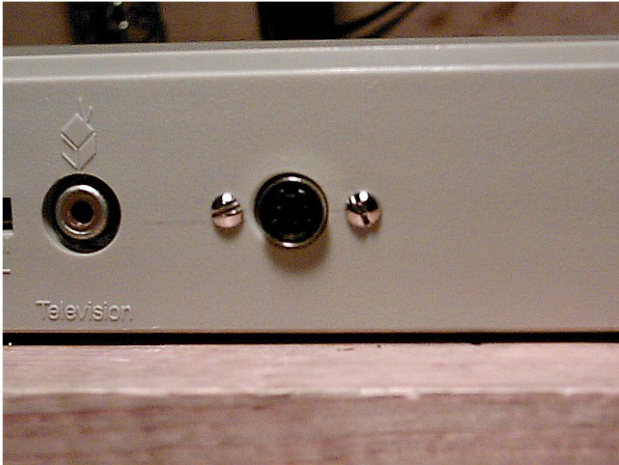
Fig5. Here is a view of the back of the XEGM with the S-video jack visible.
