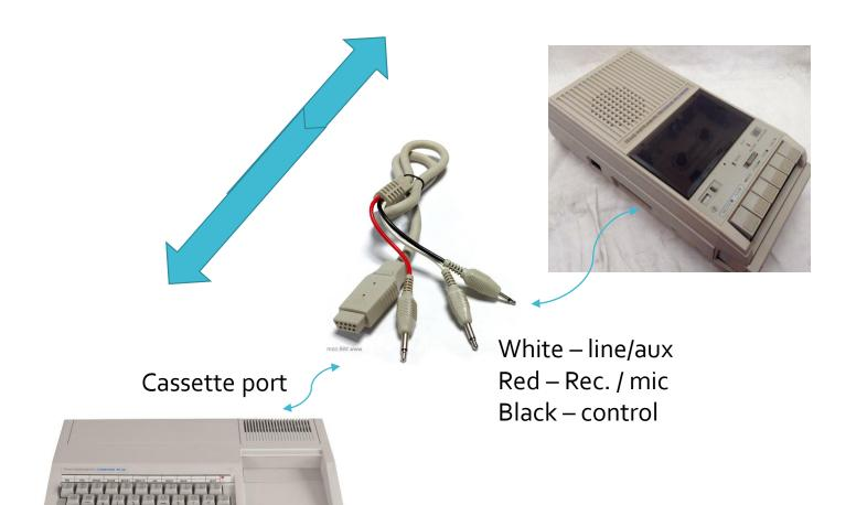
Load (OLD CS1) .wav files from PC to TI cassette port directly
