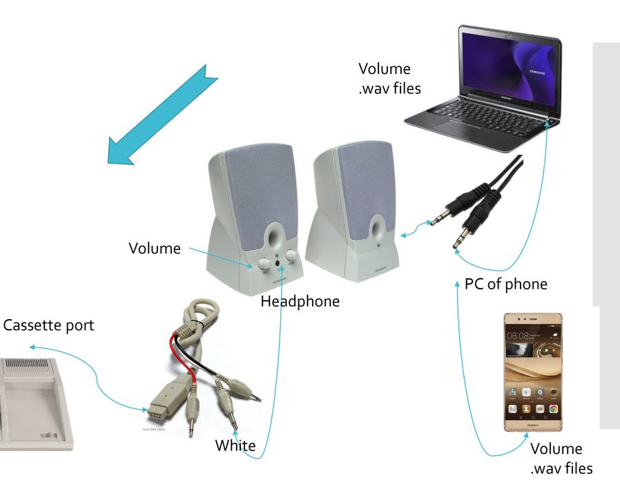
Save audio files from (any) tape recorder to a PC into .wav format (or others like .mp3)
