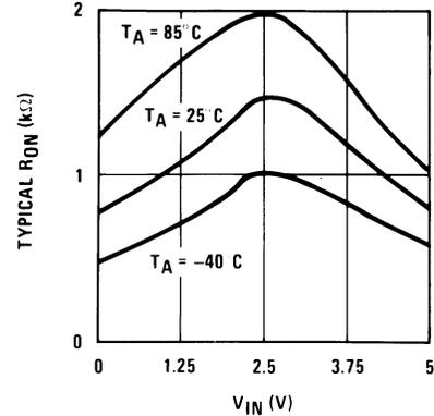
FIGURE 7. Multiplexer  $R_{ON}$  vs  $V_{IN}$
