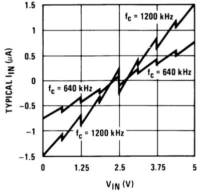
FIGURE 6. Comparator  $I_{IN}$  vs  $V_{IN}$
